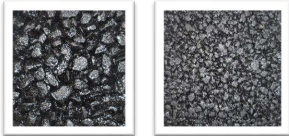
Photo-2 Conventional high-performance pavement (left) and HDULNP (right)
